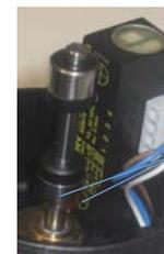
Target switch and cam for close valve
